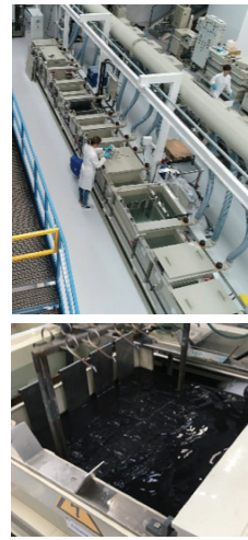
Images of the e-coating line and e-coat tank at the CIDETEC Surface Engineering facilities
